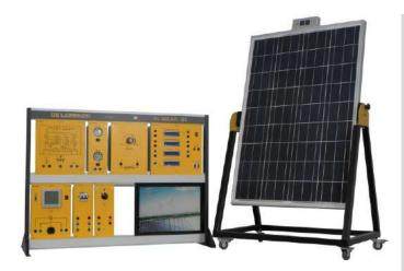
Didactic system for the study of the generation of electric energy from photovoltaic panels and its inlet in the mains network.
