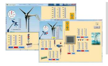
The Micro-grid Wind Turbine Trainer is supplied with a software developed in LabVIEW that communicates with the main components of the modular system via RS485 serial communication using Modbus RTU protocol to perform data acquisition and processing.
