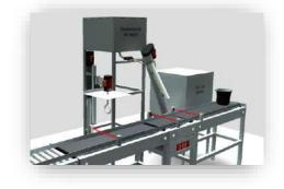
**Project:** the student is required to implement a new PLC software for the line but this time using SFC or state machine approach, in order to make it more flexible and easy to maintain. Final instructions are aimed to split the machine in 2 different state machines in order to allow simultaneous dosing and mixing operations, to increase the machine's performance.
