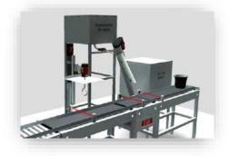
**Project:** the student is guided on the automation of the whole line using interlocks, memory, timers and dealing with the analog input to read the scale signal. He automates the sequencing step-by step in 8 tasks.
