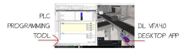
Besides DL VFA4.0 and the programming tool, there is always another software is normally open in background that is the SoftPLC. In case of Codesys, it is Codesys Control Win. If the student were using TIA Portal, the SoftPLC would be PLCSIM and if it were Rockwell the SoftPLC would be SoftLogix.
