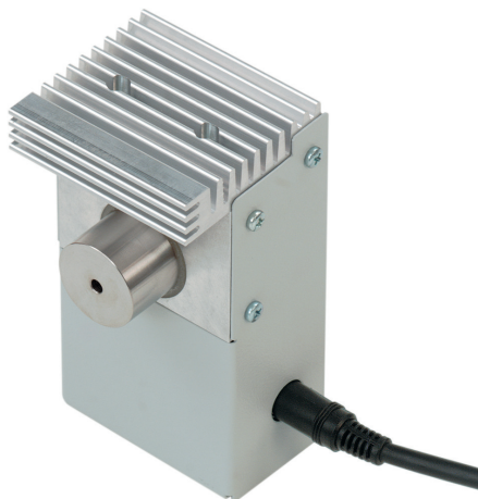
X-ray energy detector (559 938) for recording energetically resolved X-ray spectra
