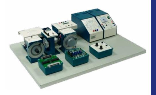
The Precision Modular Servo Workshop has been designed to give a rapid and direct path from control system design to hardware implementation. The resolution and accuracy of the system, and the consistency of its performance, makes the Precision Modular Servo Workshop ideal for serious study of digital linear servo control systems.
