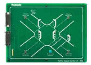
The traffic light system's simple sequence application allows control of a crossroads to be implemented on a time sequence basis. The control program can be further developed to cope with interrupts generated from pedestrian crossing requests or off-peak vehicle detector inputs.
