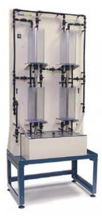
The Coupled Tanks set-up is a model of a chemical plant fragment. Often tanks are coupled through pipes and the reactant level and flow has to be controlled. The Coupled Tanks experiment is designed so that the system can be configured.
