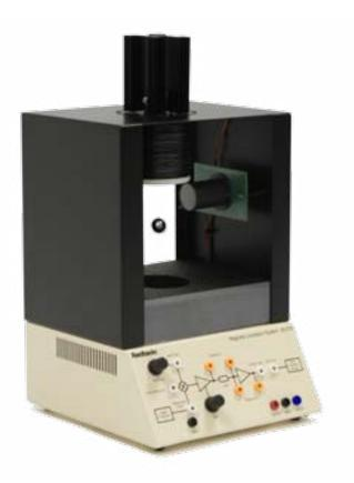
This classic magnetic levitation control problem is now presented in a new and innovative form. A 25 mm diameter, hollow steel sphere is suspended in space with visually appealing results and convenient time constants.
